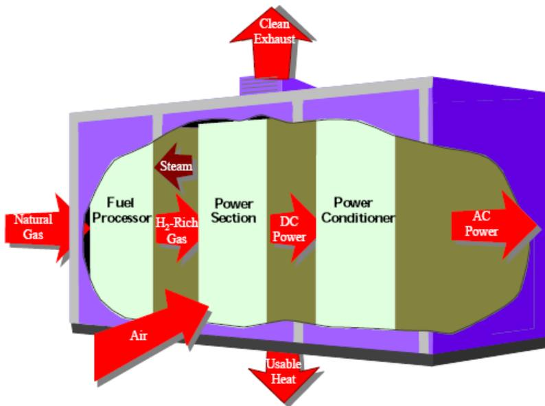
**Figure 3: Schematic view of a generic fuel cell system (Source: Gasik 2008)**
